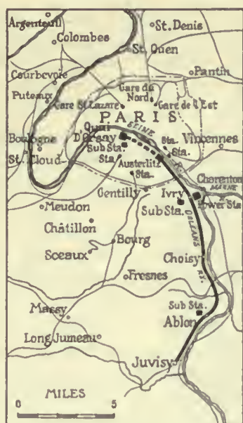
FIG. 466. ELECTRIFIED LINES OF THE ORLEANS RAILWAY
